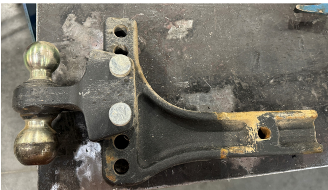
Example of an adjustable Hitch ball mount
