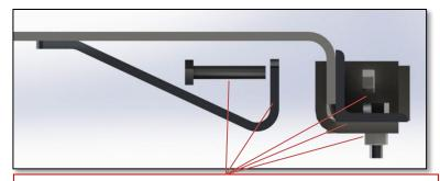
Attach reinforcing bracket, and the door bracket to rear lip of the door and the reinforcing angle to the front lip of the door with  $3/8" \times 2$  bolts and nuts on both sides. Finish attaching the door brackets using  $3/8" \times 1 \%"$  bolts and nuts.
