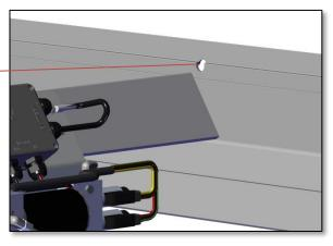
vi. Using a fish tape, pull 031-58992 – Red 4AWG x 32 feet long power wire through <u>passenger</u> side rail and through the 3/4" hole that was drilled by the control box.
