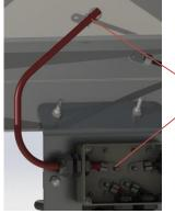
031-50504 – red 4 gage x 28 foot power wire with ½" wire loom installed on it, pulled thru the side rail and attached to the "+" terminal on the back of the control box.
