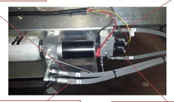
Rear hopper 029-51459 – 197" hydraulic hose. Opposite end with 90 degree fitting attaches to cylinder tube end.
