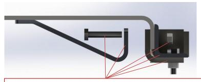
Attach reinforcing bracket, and the door bracket to rear lip of the door and the reinforcing angle to the front lip of the door with 3/8" x 2 bolts and nuts on both sides. Finish attaching the door brackets using 3/8" x 1 1/4" bolts and nuts.
