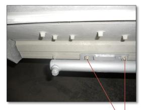
Install hydraulic cylinders with the 3/8" X 2 bolt – washer – roller – washer – washer – trap frame – cylinder foot – washer – nut.
