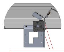
Line up leading edge of bracket with the hydraulic pump mount bracket.
