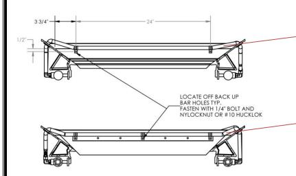
Use 029-53991 – 56-1/2" hydraulic hose. The hose goes thru the previously drilled holes and across hopper to other cylinder. Rear of hopper, cylinder rod end.
