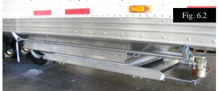
3. Locate the universal joint and roll tube spline on the tarp roll rube, rear of the trailer.
