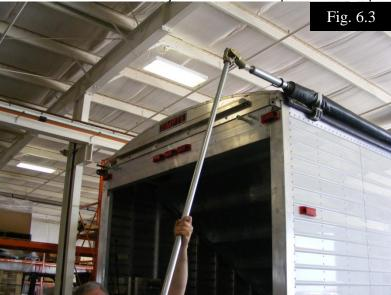
4. Slide the Tarp Crank Handle universal joint and roll tube drive spline together (rear of trailer) by pushing the universal in-place until fully engaged with the roll tube spline.
