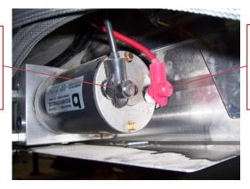
Connect red wire of wiring harness 031-50470 to terminal "2" on the hydraulic pump.
