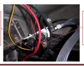
Connect the plug with red/green wires of wiring harness 031-50470 to the upper valve on the hydraulic blocking valve.
