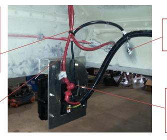
Drill 7/16" hole and connect wire as described in step g-i.
