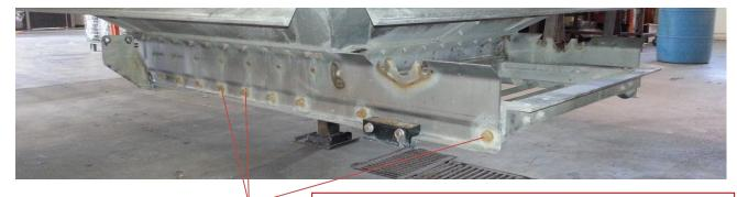
Remove these door rollers and fasteners, three per side rail.
