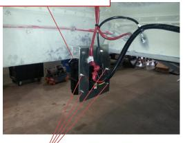
Mount control box with  $\frac{1}{4}$ " bolts and  $\frac{1}{4}$ " nylock nuts.
