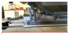
**Front hopper** 029-51239 – 104" hydraulic hose 40'/42' trailer. End with 45 degree fitting attaches to cylinder rod end.
