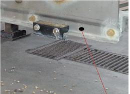
Remove the cylinder and drill hole in the trap frame rail where marked
