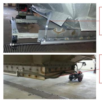
Use 029-53989 – 46-1/2" hydraulic hose. Hose goes across hopper to other cylinder. Use clips to mount as shown. Front of hopper, cylinder rod end
