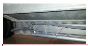
**Rear hopper** 029-51242 – 176" hydraulic hose 40'/42' trailer. End with 90 degree fitting attaches to cylinder rod end.
