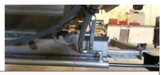
**Rear hopper** 029-51241 – 152" hydraulic hose 40'/42' trailer. End with 45 degree fitting attaches to cylinder tube end.
