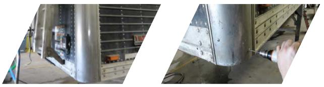
3. Drill out and remove the seven 5/16-inch rivets that connect the top rail to the corner radius.
