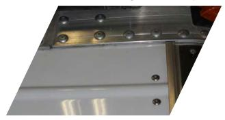
5. Remove (2-3) 3/8-inch magnaloks that connect the corner radius to the lower rail.
