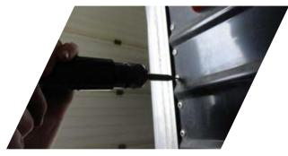
7. Remove the magnaloks on the inner liner if trailer has one in the nose.
