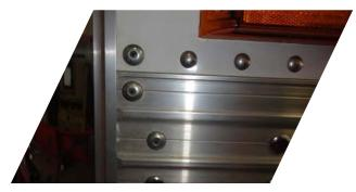
6. Remove all 1/4-inch SS magnaloks on the sidewall connected to the corner radius.
