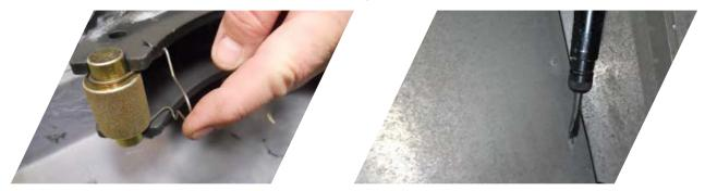
6. Install the retainer spring on the spring retainer pins on shoes before installing onto the axle.
