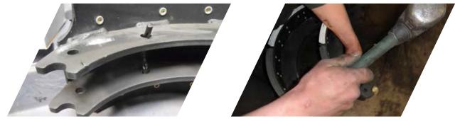
5. Install roller retainer and knurled rollers. (One per shoe)
