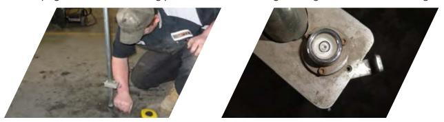
2. Place one alignment wheel cone on each side of the front axle using three of the bolts that hold the hubcap.
