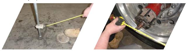
4. Attach the pull scale to the end of the tape measure. (This is used to ensure you are pulling back on the tape with the same amount of pressure on both sides of the axle.)
