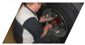
3. Attach one end of the 100-foot tape to the tab on the pogo stick and pull straight back to one of the wheel cones you placed on the front axle.
