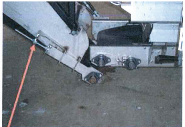
Incline conveyor tensioning bolts
