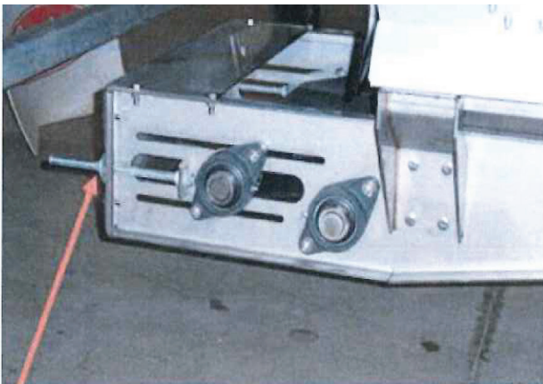
Horizontal conveyor tensioning bolts
