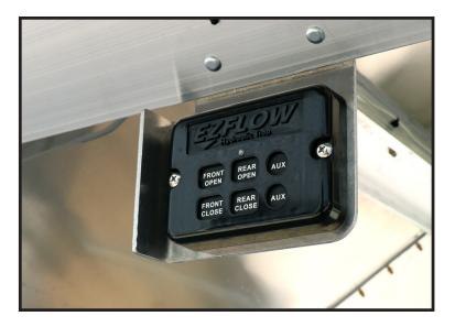
New Standard Remote allows for the operator to directly choose door open/door close. This new feature makes selecting the correct function quick and easy.
