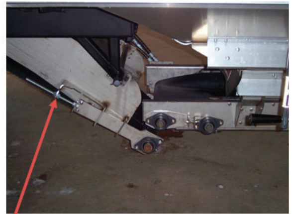
Incline conveyor tensioning bolts
