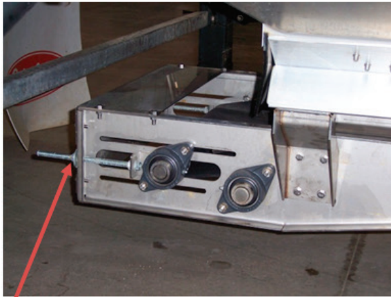
Horizontal conveyor tensioning bolts
