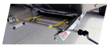
In the event of an emergency due to electrical or mechanical failures the EZ Flow<sup>XR</sup> doors can be easily converted into manual operation. The emergency manual override utilizes quick release pins and straps to open the door. This new override system is not only easy to use, but provides additional ground clearance compared to previous override systems.
