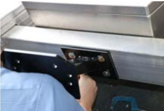
Next, place the fabric spacer onto the trailer and cover with tire mount. Line up mount/spacer with pre-drilled holes and place a 3/8 fasteners into each hole. The mount should be visually centered and cover most of the A-frame area.
