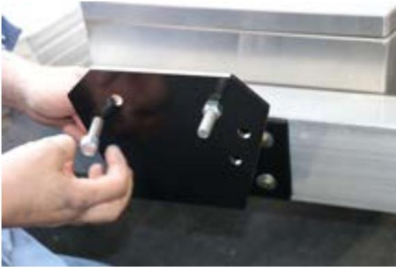
On the upper section of the tire mount, place your two 1/2" bolts (bolt head will face the trailer) and tighten for tire placement.
