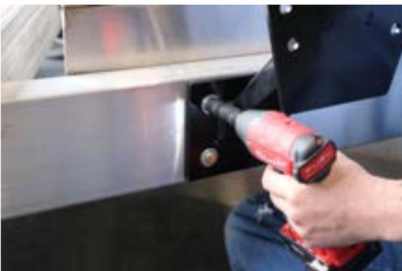
Tighten fasteners using your 9/16 socket and impact drill or ratchet wrench. Complete tightening of all four bolts moving in a clockwise manner to secure tire mount to
