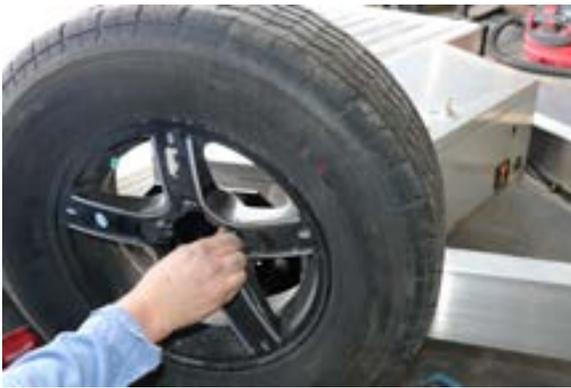
Place spare tire onto mount and fasten 3/4 bolt with a socket until tight to secure the tire.
