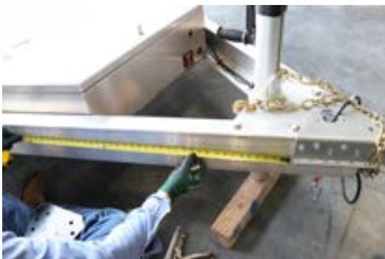
On the curbside of the trailer, take your tape measure and measure 32 1/2" from the edge of the coupler (as shown in picture), and mark a hole approximately 2" from the top edge of the A-frame. Measure a second hole 3" below your first. The third and fourth holes will measure 36 1/2" from the coupler (4" from the first set of holes) and will also be 3" apart. Once complete, the tire mount can be used to verify the marked holes are in the correct locations.
