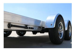
2) Release safety lever from locked position on the driver side of the trailer.
