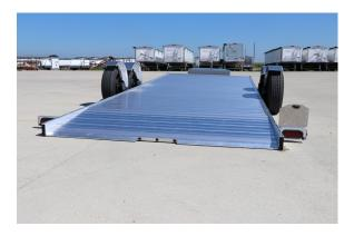
6) Lower the trailer until rear is on the ground.
