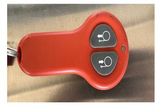
4) Press and hold the raise and lower buttons until the lights turn on. Once remote has been activated, press the lower button (arrow pointing right) and hold to lower.
