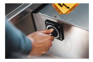
1) Unlock tool box then turn on the internal master switch to activate power and operate the hydraulic pump.
