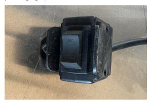
5) If preferred, trailer can be lowered using the switch located in toolbox by pressing the down button.
