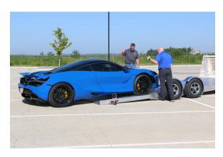
1) Roll or drive equipment onto the trailer as far forward as possible. Ensure that at least 10% of the total weight is towards the front of the trailer.
