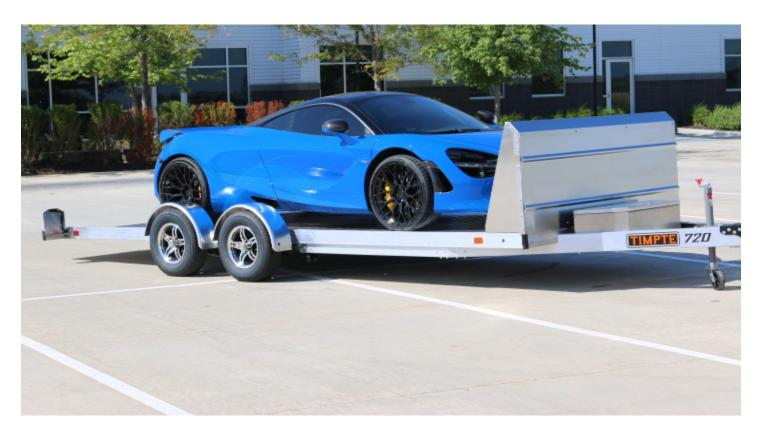
Timpte Equipment Trailers are designed specifically for carrying a variety of equipment. It is recommended that wheel tie straps be used to secure the load with the tie straps connected to the tie-downs. The load must be placed as far forward on the trailer as possible so the loaded tongue weight is 10% of the total load. Do not load cargo in the towed vehicle once it is on-board the trailer, as this may change the load distribution and overload the trailer.
