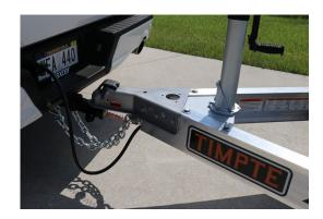
Connect the tow vehicle. Ensure the safety cables and the breakaway cable are securely connected to the tow vehicle. Safety cables must be crossed under the hitch.
