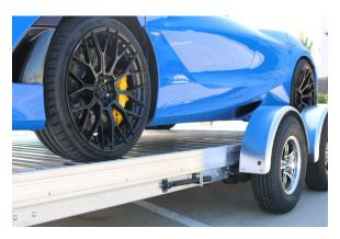
3) Latch safety lever into locked position.
