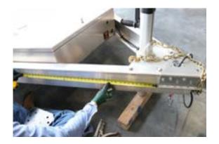
On the curbside of the trailer, take your tape measure and measure 32  $\frac{1}{2}$ " from the edge of the coupler (as shown in picture), and mark a hole approximately 2" from the top edge of the A-frame. Measure a second hole 3" below your first. The third and fourth holes will measure 36  $\frac{1}{2}$ " from the coupler (4" from the first set of holes) and will also be 3" apart. Once complete, the tire mount can be used to verify the marked holes are in the correct locations.
