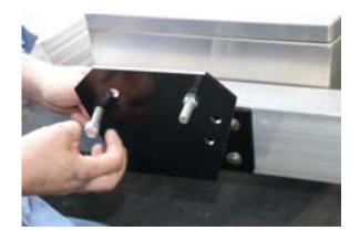
On the upper section of the tire mount, place your two %" bolts (bolt head will face the trailer) and tighten for tire placement.
