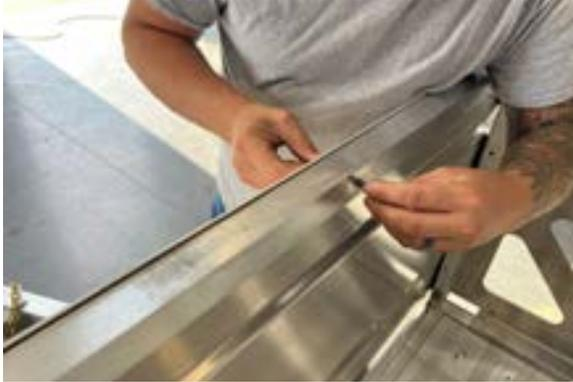
Attach your front cross member to the rock guard by inserting four 2 1/2" bolts from the outside in, and fasten loosely using 11/16" wrench.
