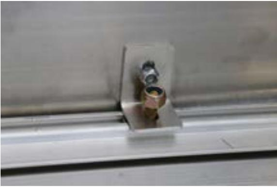
Place tire rack side panels and front panel from the rock guard kit onto the L-track studs and loosely fasten using 1/2" wrench.
