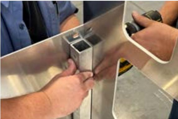
Place your two side posts and insert four 2 1/2" bolts through the four middle slots on the posts, fasten loosely using your 11/16" wrench.
