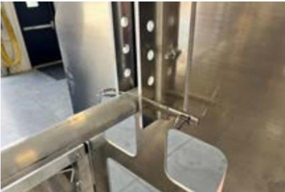
Install the upper cross member using the clevis pin.
