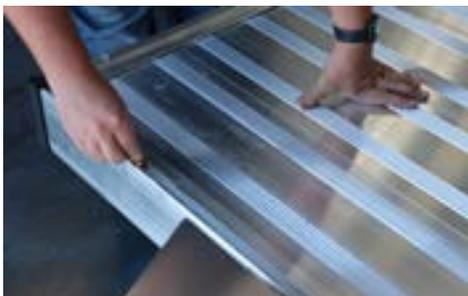
Place L-track studs into predrilled slots, 2 on each side of the trailer and 4 on the front. Discard L-track washer.
