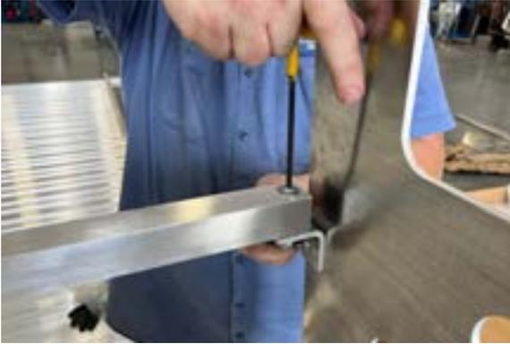
Install 1 L-bracket onto each side panel using the 1" bolts and fasten using 3/16" allen wrench. Next, install the rear cross member using the 2 1/2" bolts and fasten using 3/16" allen wrench.
