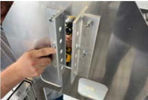
Install cross member brackets on the inside of the tire rack side panels by placing six 1" bolts in the pre-drilled holes from outside in, on each side. Fasten all bolts using 3/16" allen wrench.
