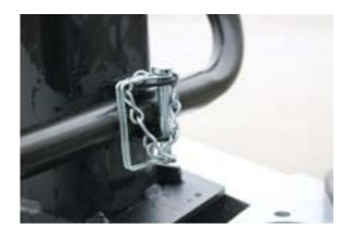
Release the jack handle by unhooking safety pin from jack.
