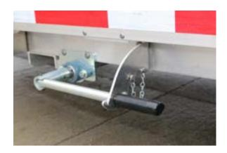
Once equipment is loaded, place the safety lever back into it's original postion and put safety pin back in to remain locked.
