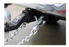
Next, attach the trailer safety chains to the tow vehicle.
