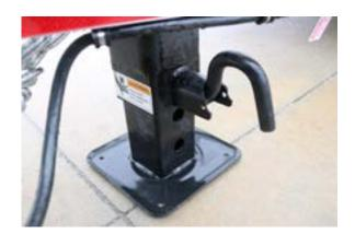
Once weight is off of the jack, pull lower jack lever to raise jack plate all the way up. (Keep fingers out of the way of jack plate).
