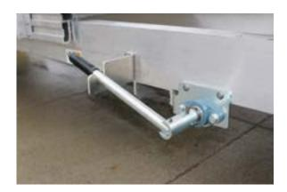
Next, release safety pin on the safety lever and place in forward facing position to allow the trailer to lower to the ground.
