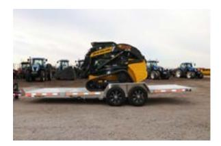
Drive equipment slightly passed the front axles to have proper load distribution on trailer.
