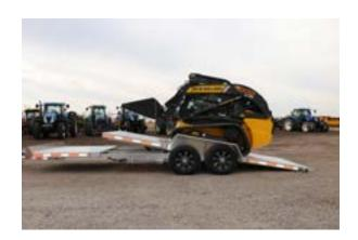
When loading your equipment make sure to raise the buckets to ensure you do not hit the trailer.
