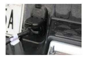
Connect the trailers electrical hookup to the tow vehicle.
