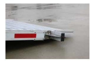
Before loading, push down on rear side of the trailer to lower the deck to the ground.
