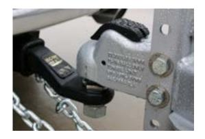
Connect the tow vehicle to the trailer using a 2 5/16" hitch.
