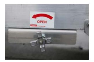
If needed, adjust hydraulic pressure on road side of the trailer to allow trailer to lower easier.
