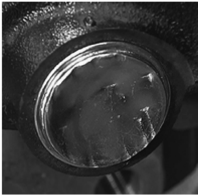
Figure 4: Damaged guide pin cap
