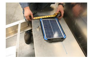
Place your solar panel in the middle of the toolbox and measure 9.5" from front side of the toolbox.
