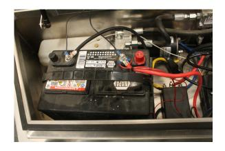
Next, place electrical connectors onto the electrical studs that are connected to the battery and fasten down.
