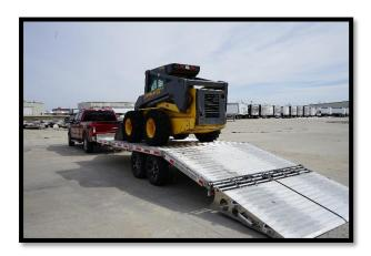
When loading your equipment make sure to raise any attachments to ensure you do not hit the trailer.
