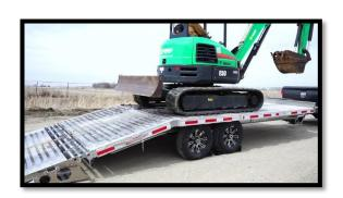
Position load so 10-15% of total load is on coupler. Proper weight distribution is **IMPORTANT**.
