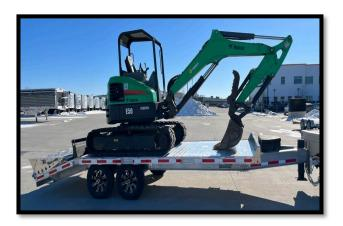
Once equipment is loaded, lock both ramps in vertical or horizontal transport position.
