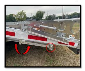
Ensure lock mechanism is engaged and pull manual ramp lock lever towards the rear of the trailer, install clevis pin.
