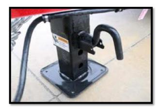
Once weight has been transferred to hitch, pull lower jack lever to raise jack plate all the way up. (Keep fingers out of way of jack plate).
