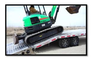
Load equipment in a safe and controlled manner to avoid damage to trailer and equipment.
