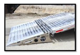
Before loading, unlock both ramps and place in the loading position.
