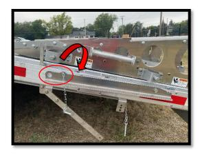
Disengage lock arm by removing snap ring and sliding lock arm off pin.
