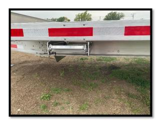
To reinstall step, pull up on step rung and push towards trailer. Ensure slide tube locks into place.
