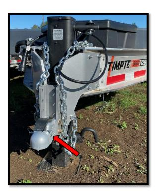
With the tow vehicle park brake engaged, connect the tow vehicle to the trailer and install the provided hitch pin.
