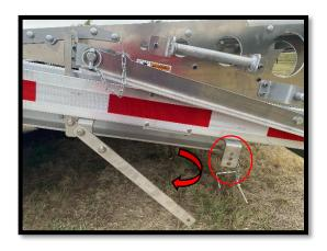
Disengage ramp lock by removing clevis pin and pulling manual ramp lock lever towards the front of the trailer.
