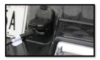
Connect the trailers electrical hookup to the tow vehicle.
