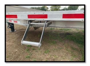
Grab step rung and pull towards outside of trailer. Ensure slide tube locks into place.
