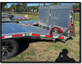
Place ramps in vertical or horizontal locking position. Install lock arm on pin and reinstall snap ring.
