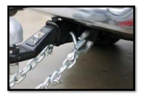
Next, attach the trailer safety chains to tow vehicle. Cross chains underneath hitch and coupler with enough slack to permit turning and to hold tongue up if the trailer comes loose.
