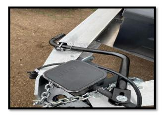
Release the jack handle by unhooking safety pin from jack.
