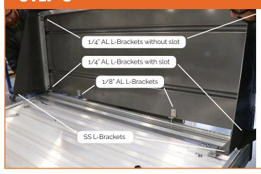
Move the Rock Guard to the trailer and attach the (6) L-Brackets to the L-Track studs using washers and tighten nuts.
