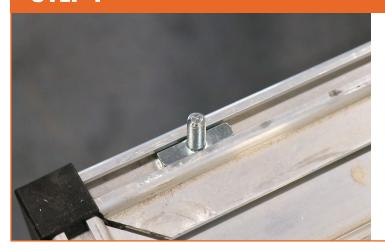
Install (1) L-Track stud in each side rail and (4) L-Track studs in the front rail of the trailer.
