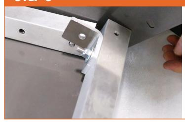
Attach an 1/4" AL L-Bracket with no slot to each side of the cross member using a 2 1/2" bolt for vertical connection.
