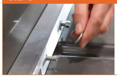
Attach 2 1/2" bolts in the (4) remaining slots on each of the corner posts.
