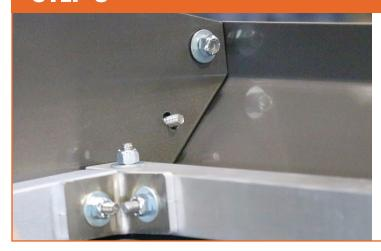
Attach the nose cone to the side panels using 3/4" bolts on the sides and 2 1/2" bolts on the front.
