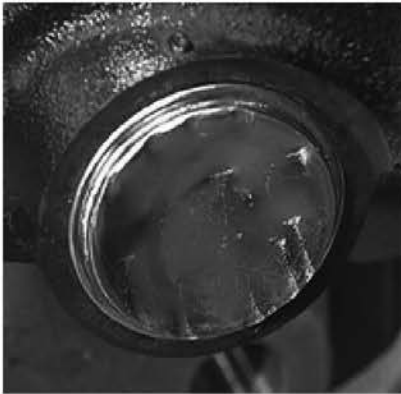
Figure 4: Damaged guide pin cap
