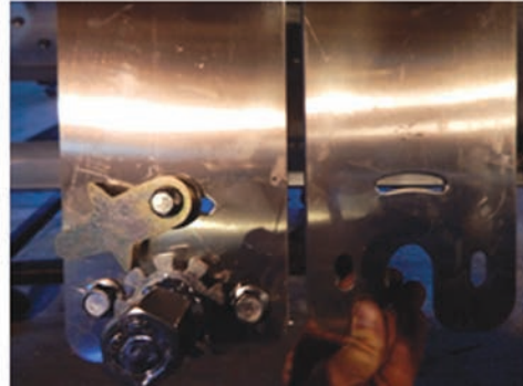
Adjustment slot (side-to-side) for torque set
