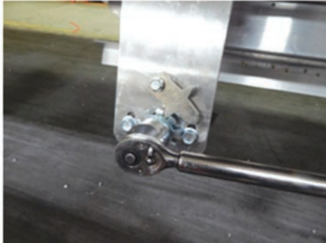
Latching Torque set to 45 ft.-lbs.
