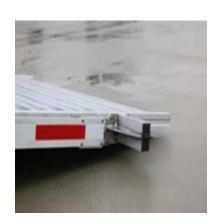
Before loading, push the rear of the trailer down until the deck rests on the ground.
