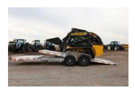
In a controlled manner, drive the equipment up on the deck. For single vehicles, the ¼ turn valve can be left in the open position. As the vehicle moves up the deck, it will begin to lower automatically. If the ¼ turn valve is in the closed position, the deck will not lower. This allows multiple smaller pieces of equipment to be loaded before lowering the deck.
