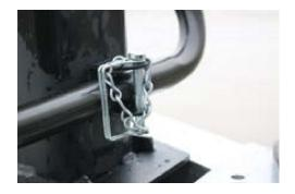
Release the jack handle by unhooking the safety pin
