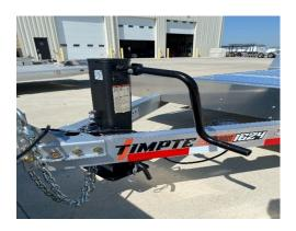
Raise the jack leg by turning the jack handle. Once the trailer is supported by the tow vehicle, pull the lower jack pin to raise the jack plate all the way up. Keep fingers clear of of the jack plate.
