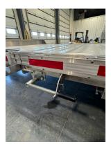
Once equipment is loaded, place the deck lock lever back into its original position and insert safety pin to ensure locked condition.
