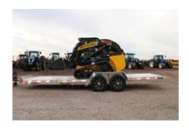
Carefully, drive equipment slightly past the front axles to have proper load distribution on trailer. 10-15% of the total load weight should be on the tongue of the trailer. Proper weight distribution is **IMPORTANT.**
