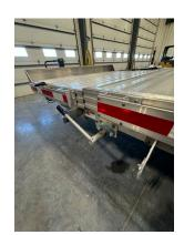
Unlock, pull out and rotate deck lock handle. Rest handle in bracket as shown.
