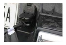
Connect the trailers electrical hookup to the tow vehicle.
