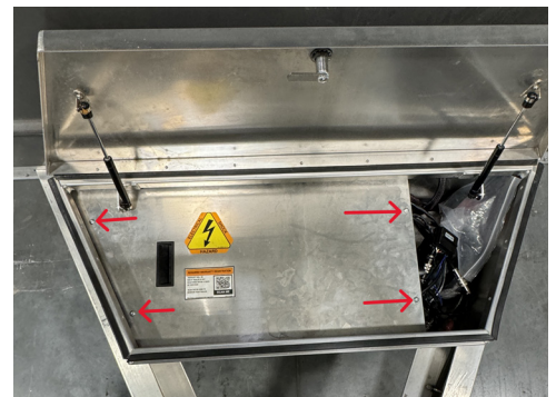
Figure 6. Battery compartment cover fastener locations.
