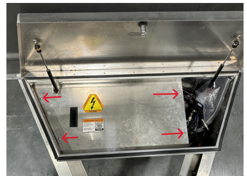
Figure 6. Battery compartment cover fastener locations.
