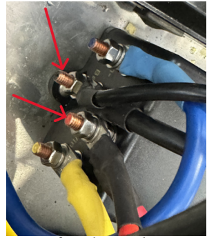
Figure 8. Lift solenoid connections
