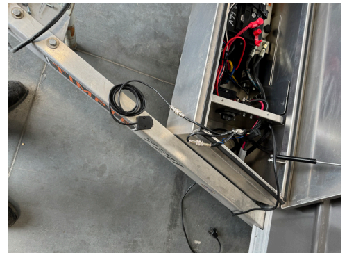
Figure 14. “Y” splitter connections
